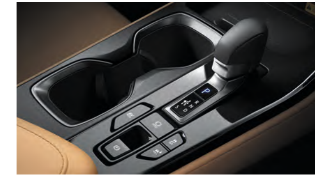
Shift lever and shift knob The shift lever is designed to provide a satisfying operating feel with gating that clicks sharply into position. With a short stroke and reduced peak load during shift operation, the lever feels light and easy to use. The shift knob was developed to provide the soft, moist feel of genuine leather, with a shape that is easy to grip and use.
