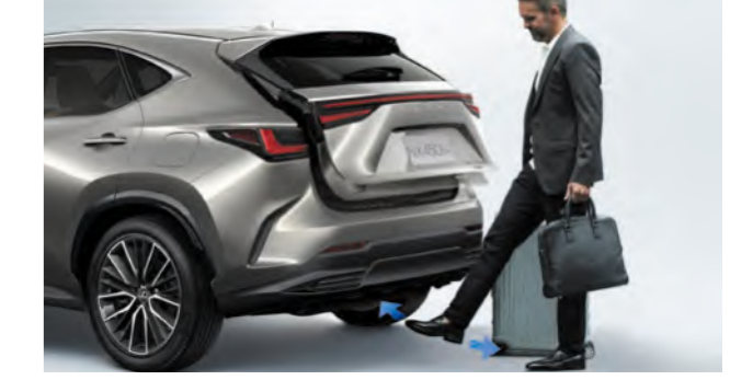
Hands-free power back door Even if both hands are full, when carrying the Electronic Key you can open and close the back door automatically by moving your foot under the rear bumper and out again. Refinements enhance fast, quiet operation, and a buzzer confirms when to move your foot out.
