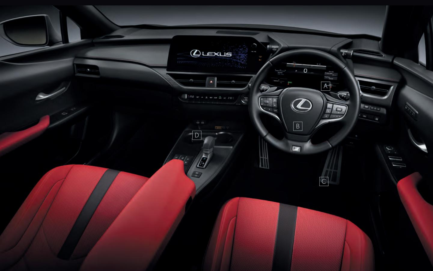
A\_Meters & multi-information display / B\_Steering wheel / C\_Aluminum pedals / D\_Shift lever knob
